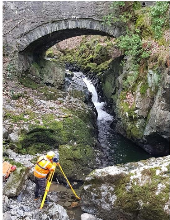
drained down however the bed levels of the deep pools were still missing which were needed to undertake accurate flood model scenarios and then design a suitable fish pass.
